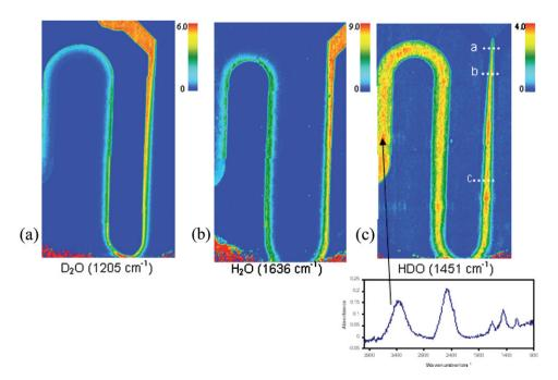
**Fig. 4** ATR-FTIR images of the microfluidic device with  $D_2O$  (left of the Y junction) and water (right of the Y junction) being introduced at a flow rate of 50  $\mu$ /hr. Images (a), (b) and (c) illustrate the flow pattern of  $D_2O$ ,  $H_2O$  and HDO in the channel respectively. The spectrum shown is extracted from the area indicated by the arrow. The overall imaged area is ~7.5 × 14 mm<sup>2</sup>.
