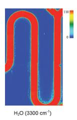
Fig. 2 ATR-FTIR image of a microfluidic channel containing water moving at a volumetric flow rate of 50  $\mu$ l/hr from each input. Red indicates a high concentration of water whilst blue indicates a zero concentration of water. The overall imaged area is ~7.5 × 14 mm<sup>2</sup>.
