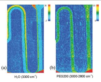
**Fig. 3** ATR-FTIR images of the microfluidic device with water (left of the Y junction) and PEG200 (right of the Y junction) being introduced at flow rates of 75 and  $25 \,\mu$ l/hr respectively. Images (a) and (b) illustrate the flow pattern of water and PEG 200 in the channel respectively. The overall imaged area is ~7.5 × 14 mm<sup>2</sup>.
