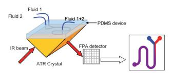
**Fig. 1** Schematic diagram of ATR-FTIR imaging system and integration with a planer, chip-based microfluidic device.
