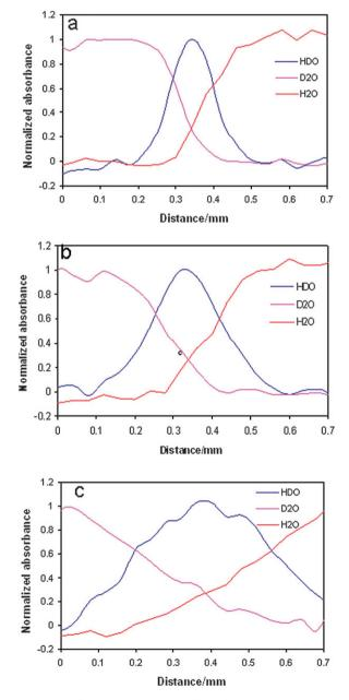
Fig. 5 Normalized absorbance profiles of  $D_2O$ ,  $H_2O$  and HDO extracted along the white dotted lines shown in Fig. 4c.
